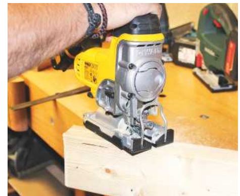
▲ Testing the saws on 90mm stock, Andy cut a basic curve
